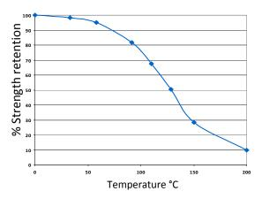
UV648 can withstand higher temperatures for brief periods (such as for paint baking and wave soldering processes) providing the joint is not unduly stressed. The minimum temperature the cured adhesive can be exposed to is -55°C (-67°F) depending on the materials being bonded.
