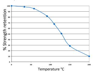
UV620 can withstand higher temperatures for brief periods (such as for paint baking and wave soldering processes) providing the joint is not unduly stressed. The minimum temperature the cured adhesive can be exposed to is -55°C (-67°F) depending on the materials being bonded.
