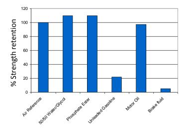
Specimens were immersed for 30 days at  $85^{\circ}\text{C}$  and tested at room temperature.
