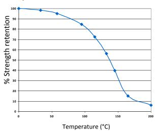
TA459 can withstand higher temperatures for brief periods (such as for paint baking and wave soldering processes) providing the joint is not unduly stressed. The minimum temperature the cured adhesive can be exposed to is -55°C (-65°F) depending on the materials being bonded.
