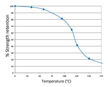
TA435 can withstand higher temperatures for brief periods (such as for paint baking and wave soldering processes) providing the joint is not unduly stressed. The minimum temperature the cured adhesive can be exposed to is -55°C (-65°F) depending on the materials being bonded.
