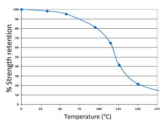
TA4300 can withstand higher temperatures for brief periods (such as for paint baking and wave soldering processes) providing the joint is not unduly stressed. The minimum temperature the cured adhesive can be exposed to is -40°C (-40°F) depending on the materials being bonded.
