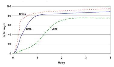
\*Cure times are typical at 23°C. Copper and its alloys will follow the faster cure while oxidised or passivated surfaces like stainless steel will tend towards the slower curve. Lower temperatures or large gaps will tend to extend the cure time. To reduce the cure time the use of Permabond® A905, ASC10, or heat can be considered.
