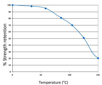
ET540 can withstand higher temperatures for brief periods (such as for paint baking and wave soldering processes) providing the joint is not unduly stressed.
