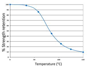
ET515 can withstand higher temperatures for brief periods (such as for paint baking and wave soldering processes) providing the joint is not unduly stressed. The minimum temperature the cured adhesive can be exposed to is -40°C (-40°F) depending on the materials being bonded.
