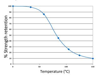
ET510 can withstand higher temperatures for brief periods (such as for paint baking and wave soldering processes) providing the joint is not unduly stressed. The minimum temperature the cured adhesive can be exposed to is -40°C (-40°F) depending on the materials being bonded.
