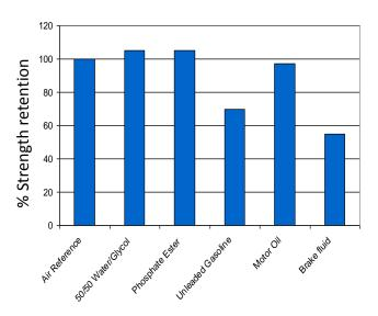
Specimens were immersed for 30 days at 85°C and tested at room temperature.
