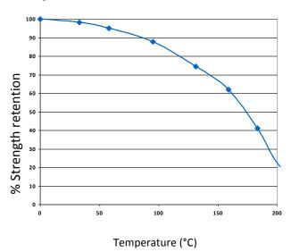
ES578 can withstand higher temperatures for brief periods (such as for paint baking and wave soldering processes) providing the joint is not unduly stressed. The minimum temperature the cured adhesive can be exposed to is -40°C (-40°F) depending on the materials being bonded.
