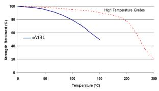
"Hot strength" shear strength tests performed on mild steel. 24hr cure at room temperature and conditioned to pull temperature for 30 minutes
