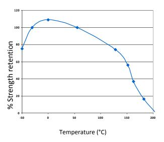
"Hot strength" shear strength tests performed on mild steel. 24hr cure at room temperature and conditioned to pull temperature for 30 minutes before testina.
