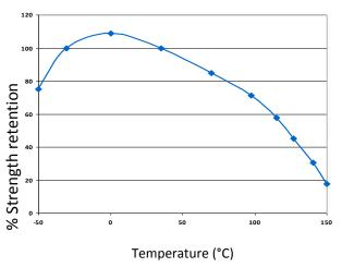
"Hot strength" shear strength tests performed on mild steel. 24hr cure at room temperature and conditioned to pull temperature for 30 minutes before testina.
