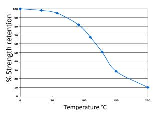
UV649 can withstand higher temperatures for brief periods (such as for paint baking and wave soldering processes) providing the joint is not unduly stressed. The minimum temperature the cured adhesive can be exposed to is -55°C (-67°F) depending on the materials being bonded.
