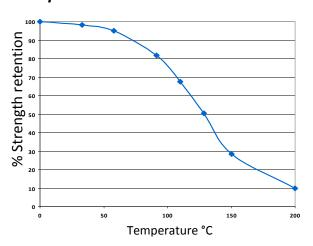
UV630 can withstand higher temperatures for brief periods (such as for paint baking and wave soldering processes) providing the joint is not unduly stressed. The minimum temperature the cured adhesive can be exposed to is -55°C (-67°F) depending on the materials being bonded.
