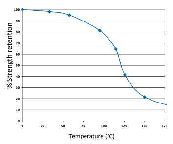
TA4246 can withstand higher temperatures for brief periods (such as for paint baking and wave soldering processes) providing the joint is not unduly stressed. The minimum temperature the cured adhesive can be exposed to is -40°C (-40°F) depending on the materials being bonded.
