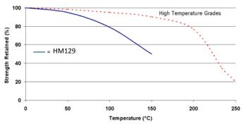
"Hot strength" shear strength tests performed on mild steel. 24hr cure at room temperature and conditioned to pull temperature for 30 minutes before testina.
