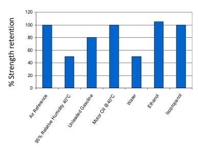
Specimens were immersed for 1000 hours at 22°C (unless otherwise stated)
