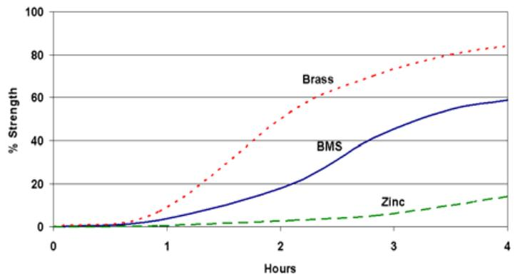
\*Cure times are typical at 23°C. Copper and its alloys will follow the faster cure while oxidised or passivated surfaces like stainless steel will tend towards the slower curve. Lower temperatures or large gaps will tend to extend the cure time. To reduce the cure time the use of Permabond<sup>®</sup> A905, ASC10, or heat can be considered.
