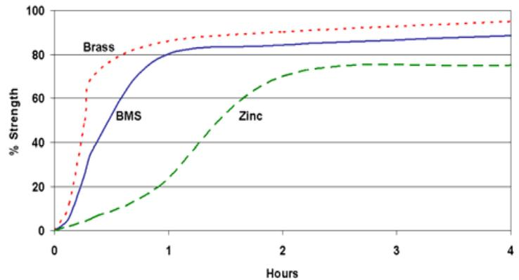
\* Cure times are typical at 23°C. Copper and its alloys will follow the faster cure while oxidised or passivated surfaces like stainless steel will tend towards the slower curve. Lower temperatures or large gaps will tend to extend the cure time. To reduce the cure time the use of Permabond® A905, ASC10, or heat can be considered.
